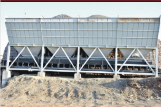
Inline Silo for Aggregate Storage
