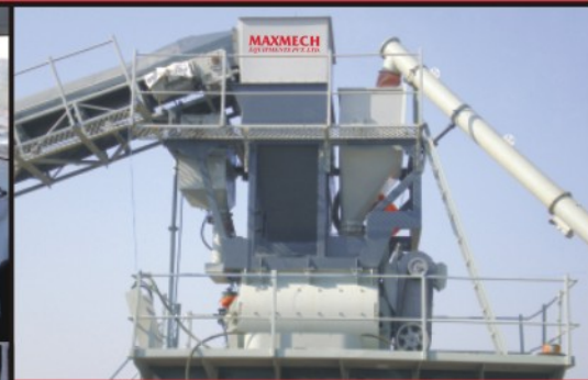
Cement & Water Weighing with Mixer Module
