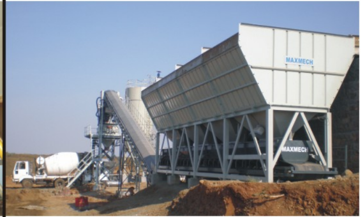
90 m 3 / hr. Plant with Belt Conveyor & Inline Silo
