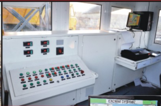
Control Panel & PC with Core 2 Duo Processor & Online Printout System with SCADA Software
